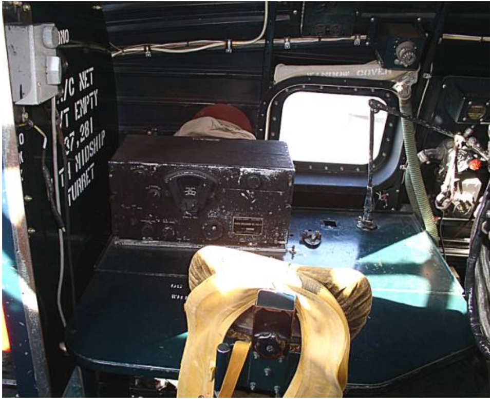
The receiver BC-348-N built by Wells Gardner seems to have been heavily used!
