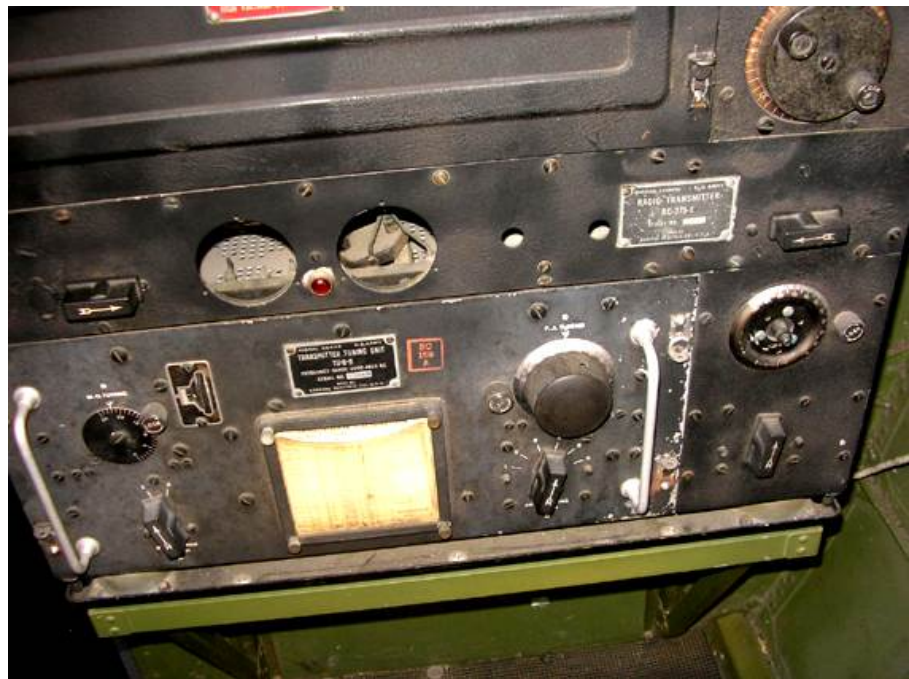
The transmitter BC-349 which was used together with the BC-348 receiver for HF communication with the home bases. Here in the Aluminum Overcast.
