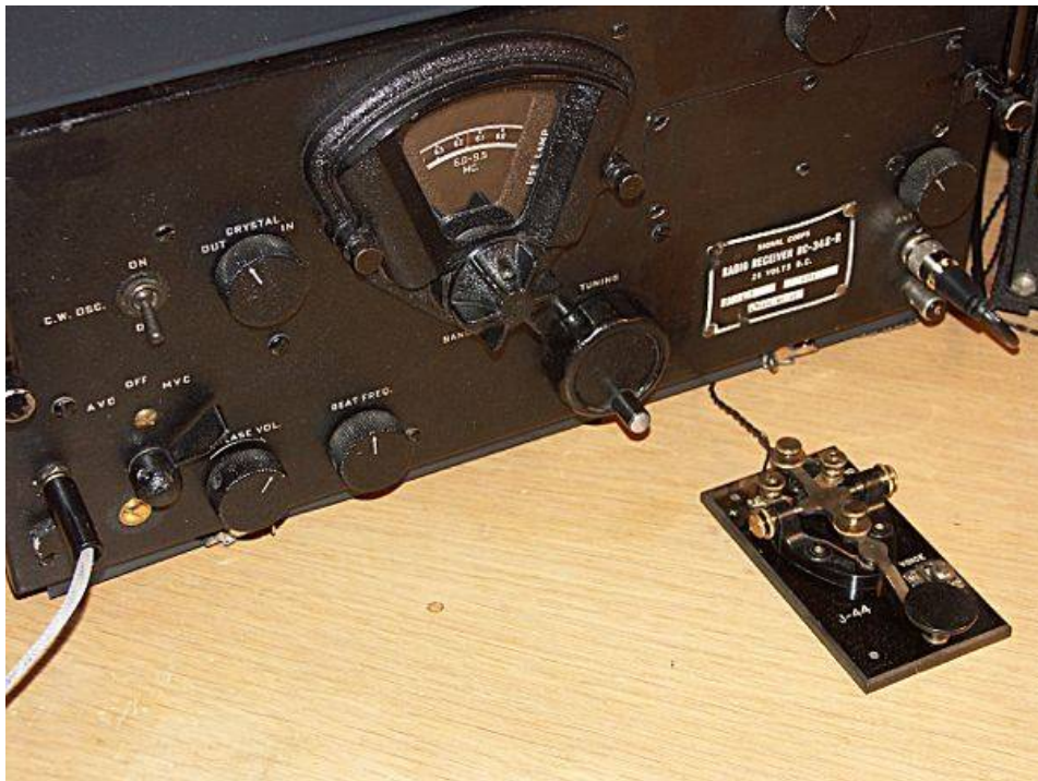
My BC-348-R with the J-44 key (before repainting the panel). The key is connected to a morse training oscillator.
